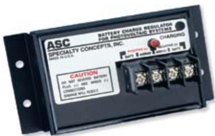
The ASC is a compact, encapsulated, battery charge regulator for use in small photovoltaic systems. It is available in 12-volt and 24-volt units up to 16 amps. The ASC is a switching shunt regulator, housed in an anodized aluminum chassis and encapsulated in a hard epoxy resin. The terminal block accepts up to 12-gauge wire or a spade connector, providing simple installation.
