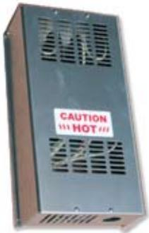
These resistive loads enclosed in vented aluminum boxes can be used in 12-, 24 and 48-volt diversion regulation systems. The aluminum box may get very hot in operation. It should be mounted on a nonflammable surface and should be at least 12" from any flammable material.
