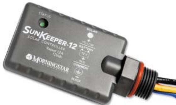
The SunKeeper is available in 6-amp or 12-amp versions at 12 volts DC. To withstand the high temperatures at the solar module, the controller has been designed using extremely efficient power electronics and is rated to 70C. The SunKeeper is also certified for use in Class 1, Division 2 hazardous locations, making it an ideal controller for solar powered oil/gas applications. Mounts in 1/2" knockout. 5-year warranty.
