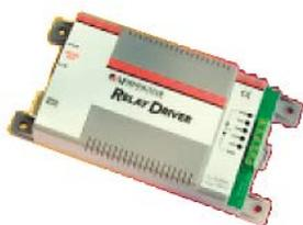
The Relay Driver may be mounted to a DIN rail and is fully programmable with the included PC software via serial RS-232 port connection. Dimensions are 6.4" x 3.2" x 1.3" and weight is 0.4 lb. Terminals can accept 16- to 24-AWG wire. Self consumption is less than 20 mA and the unit will operate from 8 to 68 volts DC. 3-year warranty
