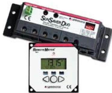
This controller includes a backlit remote meter which may be mounted in or on a wall, and displays digital and pictorial status information about the solar power system. The SunSaver Duo is epoxy encapsulated for environmental protection, is user adjustable via DIP switch or connection to a personal computer and has an optional remote temperature sensor. 5-year warranty.
