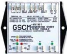
This generator start controller is optimized for use with OutBack inverters. It supports three types of 3-wire gas-generator control: momentary, maintained or ignition. It has a fixed crank time and over and under frequency shutdown.
