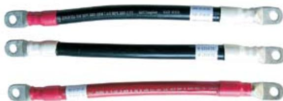
Use these cables between individual battery cells or between battery banks. Circuits protected by 250-amp breakers or 400-amp fuses should use 4/0 cables. Use 2/0 cables for 175-amp breakers and 200-amp fuses. Use #2 cables for 110-amp or smaller fuses or breakers. Cables with 1 red end and 1 black end are used for series battery interconnects. Cables with white ends are for negative battery parallel jumpers.
