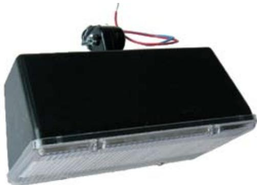
These weatherproof lights are designed to meet the demand for solar powered sign lighting and area lighting. They have ½" male pipe thread mounts and can be used for up lighting or down lighting. They use an electronic ballast that will operate down to -20 ° F. Replacement fluorescent tube is S/E 13-watt tube. This light uses 1 amp at 12VDC.
